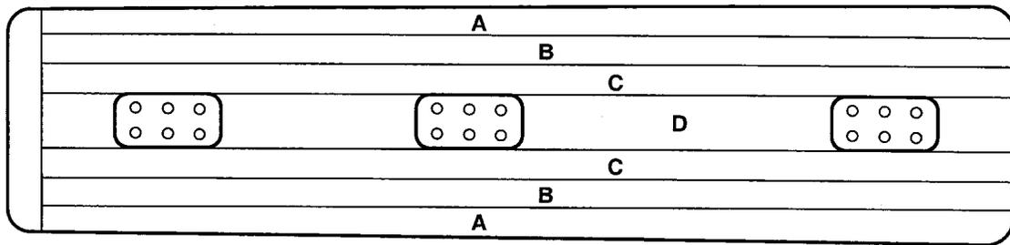
Fig. 7 Demonstrates how the flap and seal components were divided into rows for machining length-wise test specimens
