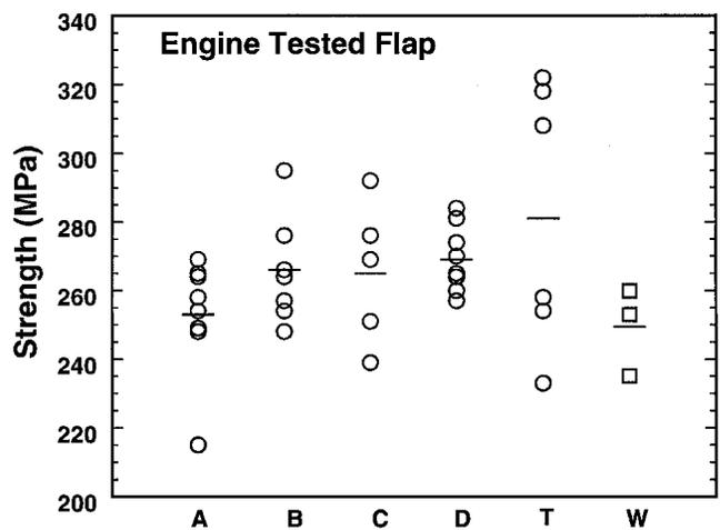
**Fig. 9** Tensile strength data generated from all test specimens machined from the engine-tested SiC/C divergent flap
