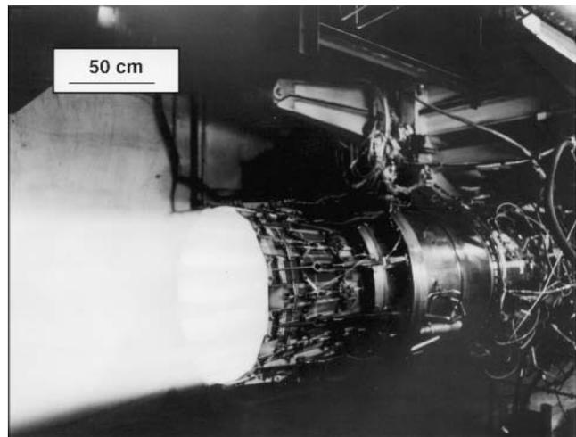
**Fig. 5 F414 ground-test turbofan engine during operation with the integrated SiC/C flap and seal nozzle configuration<sup>[3]</sup>**
