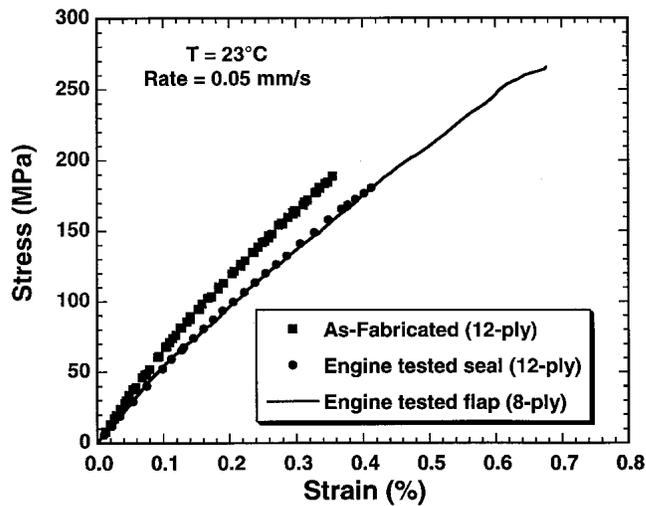
**Fig. 11** Stress-strain behavior of engine-tested flap and seal material as well as the behavior of as-fabricated 12-ply seal material<sup>[10]</sup>
