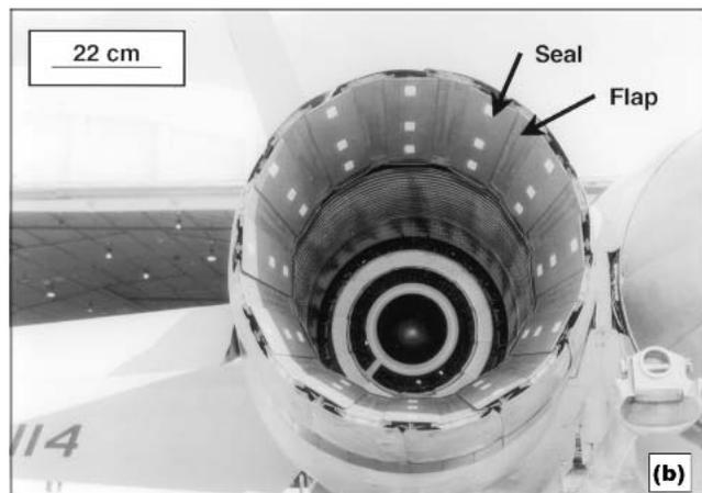
**Fig. 1** (a) A schematic of the VEN's axisymmetric pattern in which each seal overlaps the edges of the two adjacent flaps<sup>[2]</sup>; (b) a view into one of the GE F414 VENs on a Navy F-18 fighter jet
