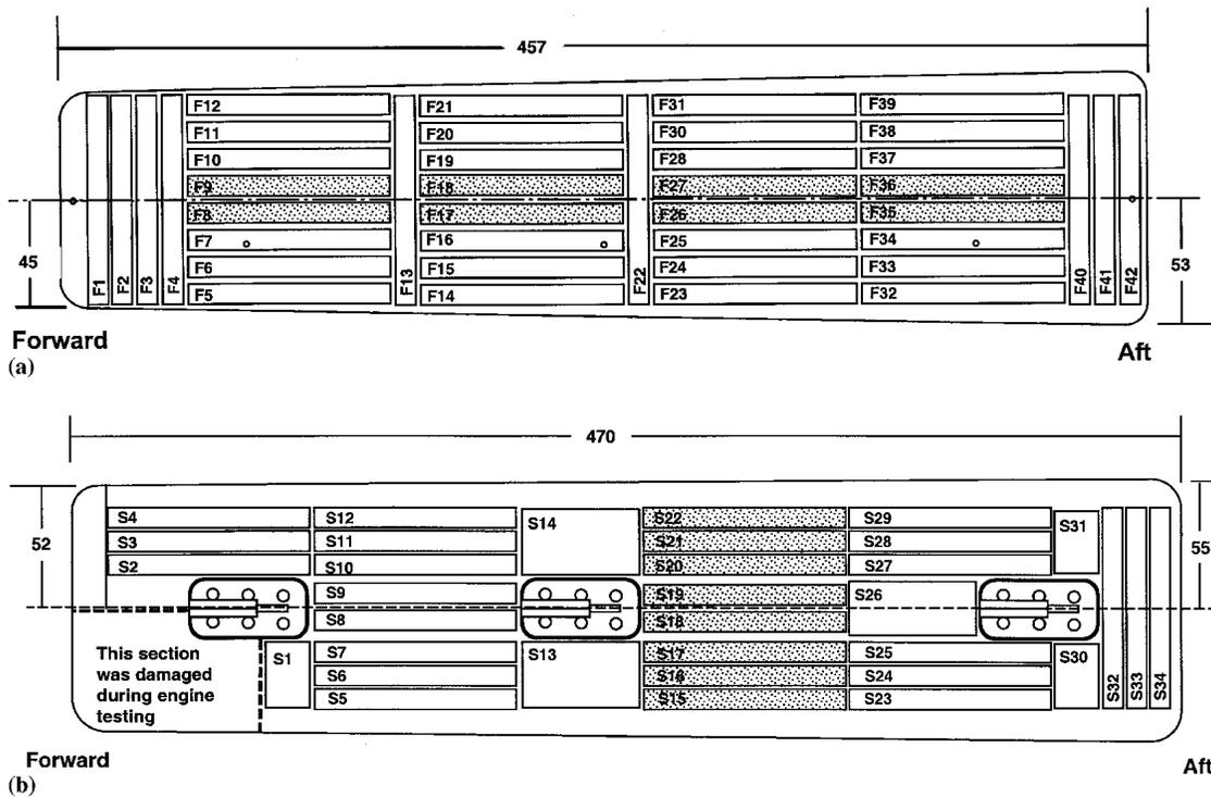
Fig. 8 (a) Specimen layout used for the engine-tested flap (specimens shown with open circles were not tension tested in this study); (b) specimen layout used for the engine-tested seal
