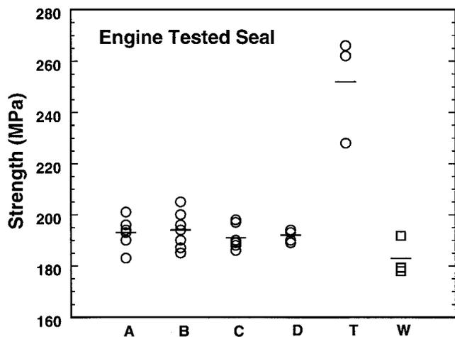
**Fig. 10** Tensile strength data generated from all test specimens machined from the engine-tested SiC/C seal
