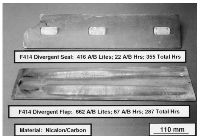
**Fig. 6** The divergent flap and seal components received from GE after being tested on an F414 ground-test engine
