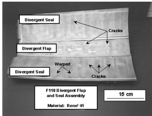
**Fig. 2** Nickel-base superalloy (Rene' 41) exhaust nozzle components removed from an F110 engine before reaching their design life due to severe deformation and cracking
