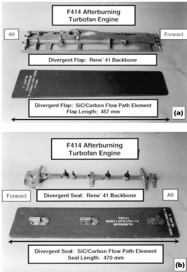
**Fig. 3** F414 VEN flap (a) and seal (b) with their respective metal hardware
